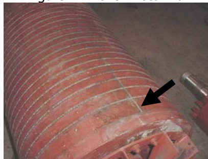
Figure 7: Broken Rotor Bar
